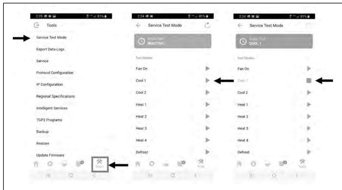
Figure 109. Symbio 700 service test mode
